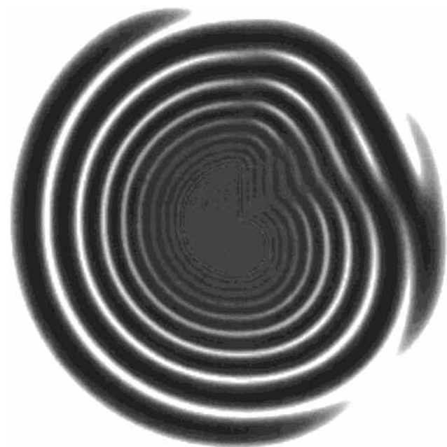
Figure 9. Simulation of a spiral system of Liesegang rings using system (2). Grayplot at t = 83:20 h. The radial symmetry breaking branch point is induced by the ragged contour of the central silver drop. Initial concentrations: a_0 = 0.7 M within the drop, b_0 = 5.14 mM throughout. Horizontal field of view: 74 mm (full simulation field: 88 \times 88 mm). Other parameters and scalings, see Figure 6.
